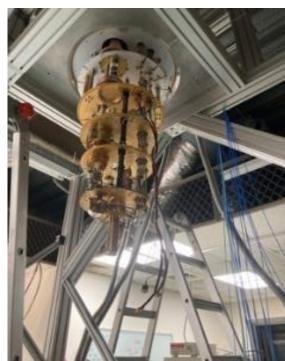
Picture of an open dilution refrigerator that can reach the base temperature of 10 mK
